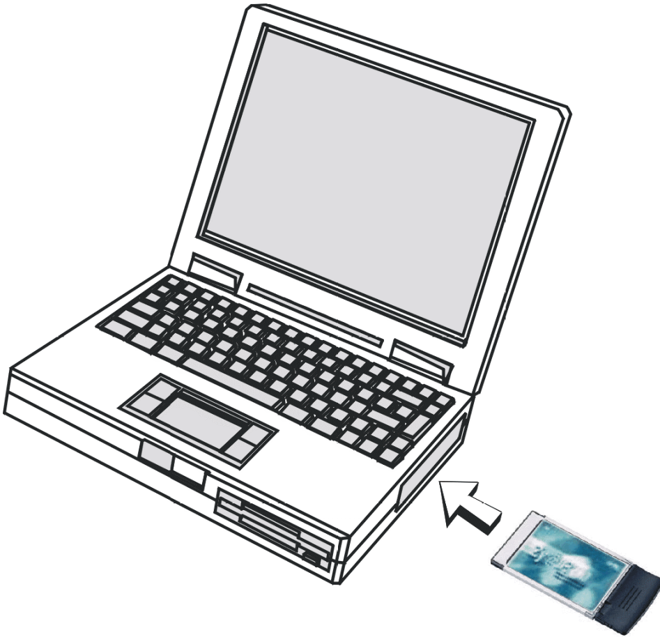
Figure 2-1 Inserting the ZyAIR 100 into the Notebook Computer
