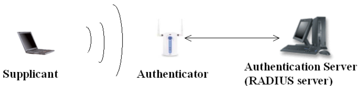
Figure 2. IEEE 802.1X w/ Standalone RADIUS server
